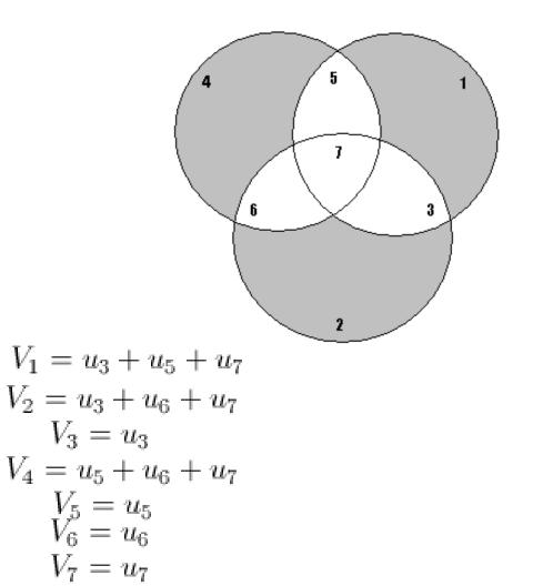
•Where  $V = (V_1, V_2, V_3, V_4, V_5, V_6, V_7)$  is the codeword
